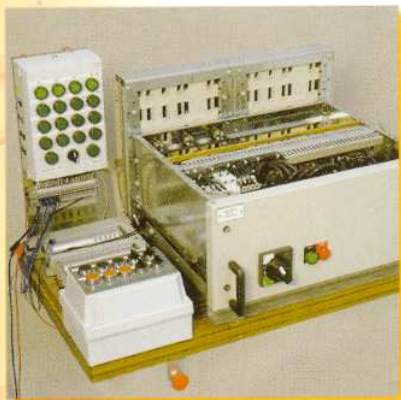
Electrical test of S4 drawers
